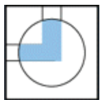
#2 90° Housing, #2 90° Plug For single right hand flow. 7011KV 7011KVP
