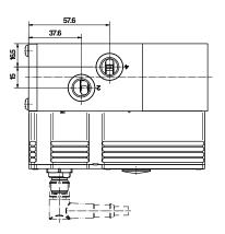
1 Valves are delivered with M4 x 50 mounting screws
