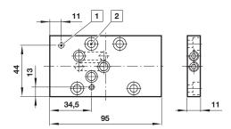
☐ Two screws M4 x 50 mm deep to mount the VP50 onto the manifold ☐ Four screws M6x16 mm deep to mount the manifold onto the iso subbase
