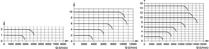
Flow rate characteristics NG 16/connection plate 3/4" (NG20); P1=7 bar, 12 bar, 17 bar
