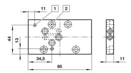
☑ Two screws M4 x 50 mm deep to mount the VP50 onto the manifold
