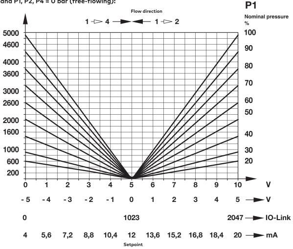
Flow-rate as a function of the pressure ratio P2/P1 for setpoint values 10, 20, ...100%
