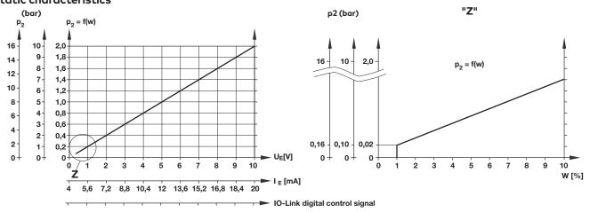
Flow rate characteristic as a function of the set-point (voltage/current/digital IO-Link) and input pressure 7 bar, 12 bar, 17 bar for nominal value 8 and 16
